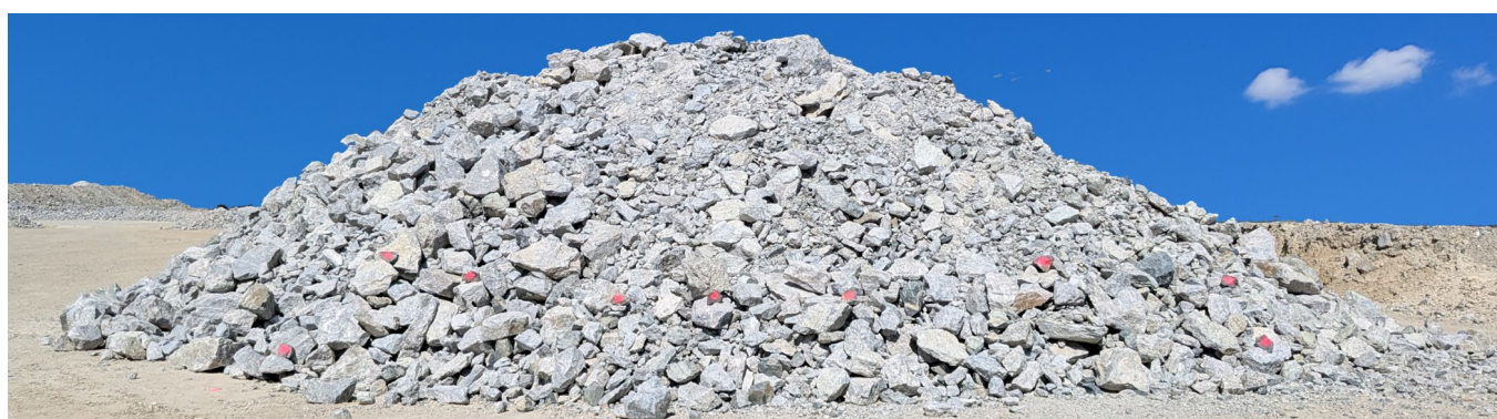
Figure 4 Close up of block tip shown basalt rocks marked with pink paint for easy visual identification
